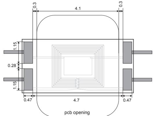
For shortest response time, in case of mounting onto a printed circuit board (PCB), HMC03M shall be positioned over an opening to allow enough air circulation around the sensor.
