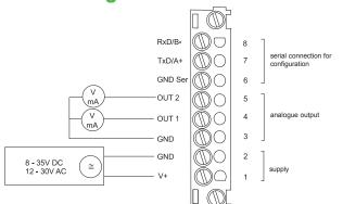
Terminal configuration - Alarm output
