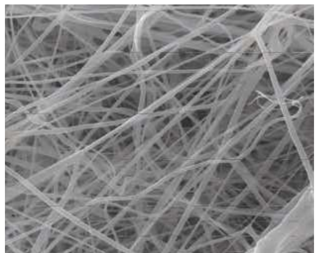
Revo II filter media photographed with an electron microscope at 2,500 times magnification
