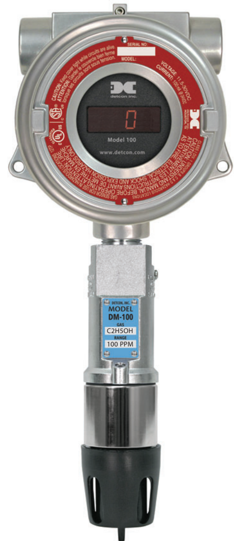
(shown as PN 961-E00022-100 in Aluminum j-box with Loop Powered Display)
